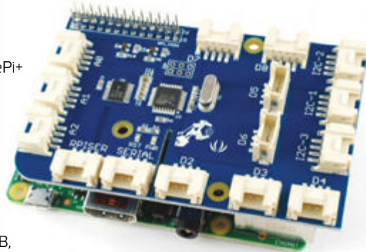
The GrovePi+ board mounts on top of any Pi, and you can still use the GPIO port for other hardware
