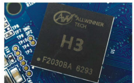
The quad-core AllWinner H3 is surprisingly capable, bettering the Raspberry Pi 2 for performance
